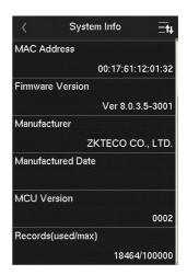
Here, you can view the device name, serial number, MAC address, firmware, manufacturer and MCU version information.
