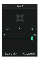
Select the zone to be adjusted, adjust the sensitivity of the zone in the zone interface, and click [Confirm (OK)] to save.
