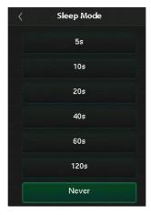
If you have activated the sleep mode, when there is no operation, the device will enter the standby mode. Press any key or finger to resume the normal working mode. You can disable this function or set the value to 5s, 10s, 20s, 40s, 60s or 120s.
