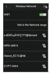
Tap on the required Wi-Fi name from the available list and input the correct password in the password interface, and then tap **Connect to WIFI (OK)**.
